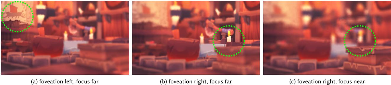
Fig. 1. *Foveated light field display and rendering.* (a), (b), (c) are our simulated retinal images under foveation with different tracked eye gazes (shown in green circles) and different focus planes. Specifically, (b) has the same gaze position but different focus plane from (c), and the same focus plane but different gaze position from (a). Our method traces only 25% of the light field rays while preserving perceptual quality.
